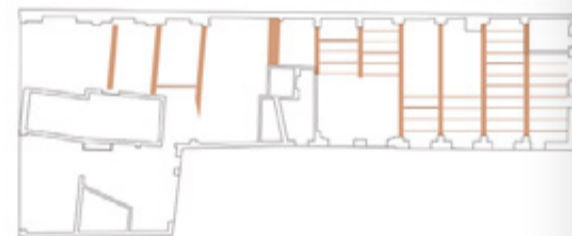
LOAD-BEARING STRUCTURE OF THE BUILDING structure, posts, beams / large, free spaces / no load-bearing walls
